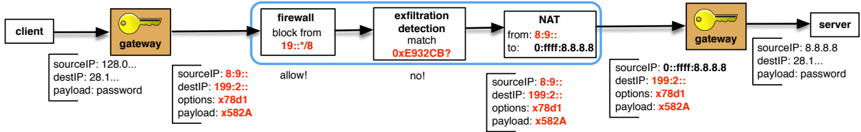
Figure 2: Example of packet flow through a few middleboxes. Red in bold indicates encrypted data.
