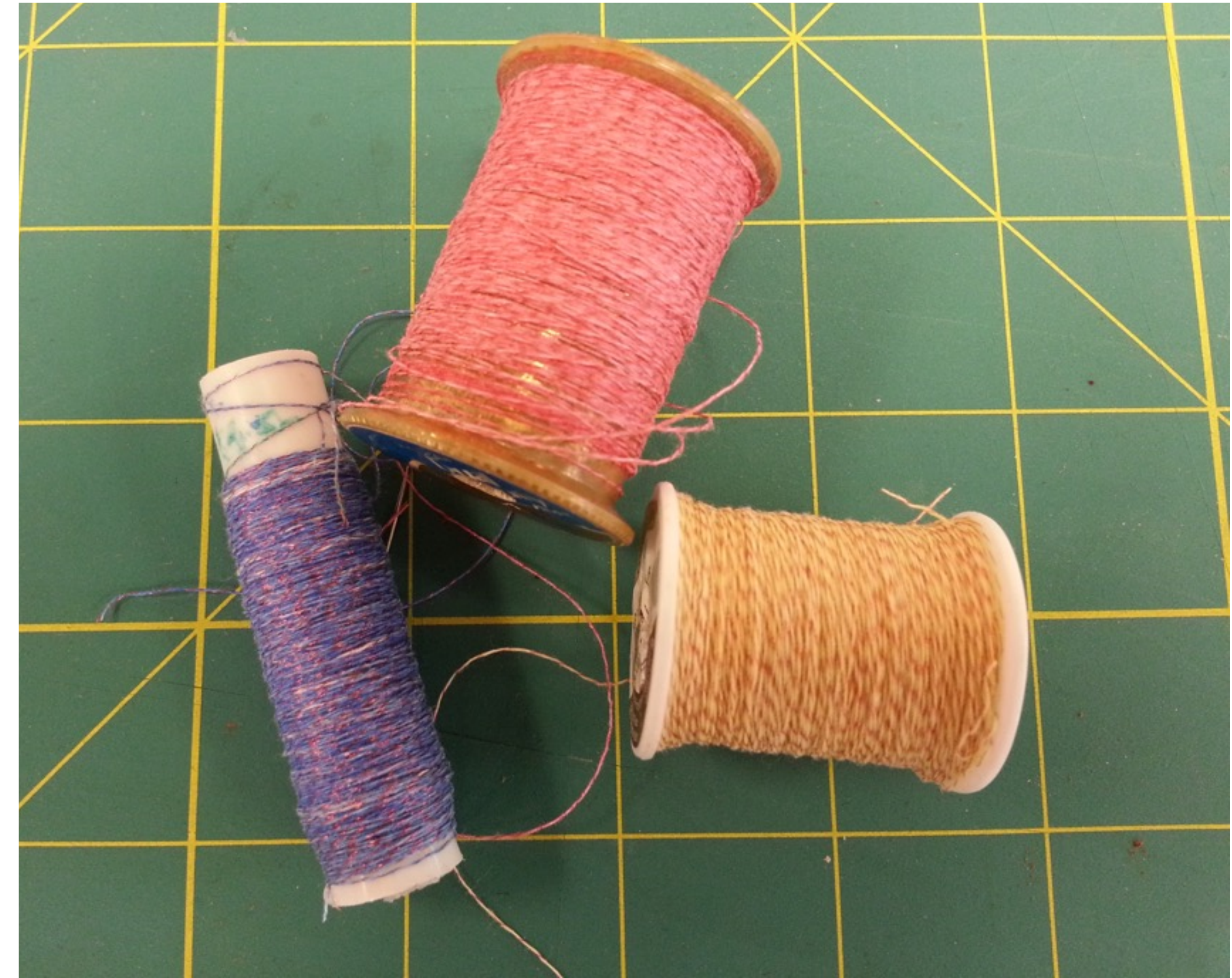
jacquard thread coated with thermochromic paint
